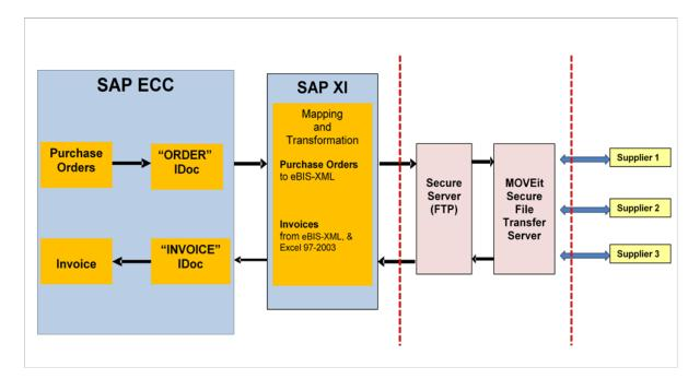
The diagram below provides a high level overview of TfL's eP2P solution
