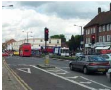
Figure 4.1: Bus advance area using pre-signals (from [16])
