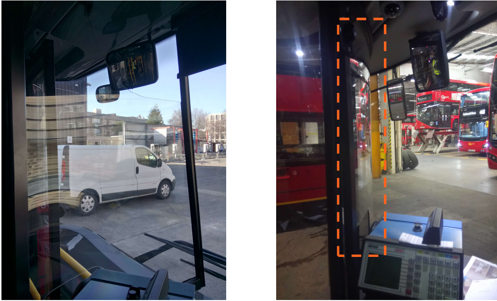
Figure 18: Partial A-pillar overlap and reflectance through a Curved Inwards Assault Screen (left). Unobstructed view of external and internal mirrors and area of optical distortion and reflectance caused by Curved Away Assault Screen (right)
