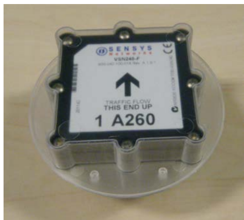
Magnetometer used as part of SCOOT installation
