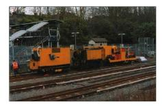
Rail grinding to restore rail profiles continues to be a successful noise reduction measure. Last year, over 20 km of track was reground or replaced. Other engineering practices, such as lubrication of curved sections, train speed restrictions in sensitive areas and better line-side vegetation management are also helping to reduce noise levels.
