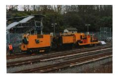
Rail grinding to restore rail profiles continues to be a successful noise reduction measure. 3 sites have been completed this year – Victoria-Brixton, Highbury-Kings Cross and Highbury-Seven Sisters. Other changes such as lubrication of curved sections, train speed restrictions in sensitive areas and better line-side vegetation management are also helping.
