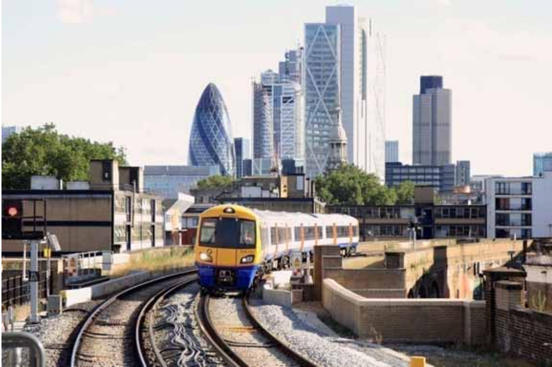
Figure 8.4 East London line Class 478 'Electrostar' electric multiple unit train approaching Hoxton station.
