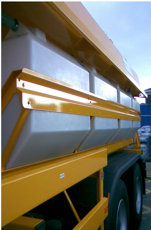
Figure 4.1 Modified Gritter Vehicle showing pre-wet tanks (left hand side) and application dish (right hand side)
