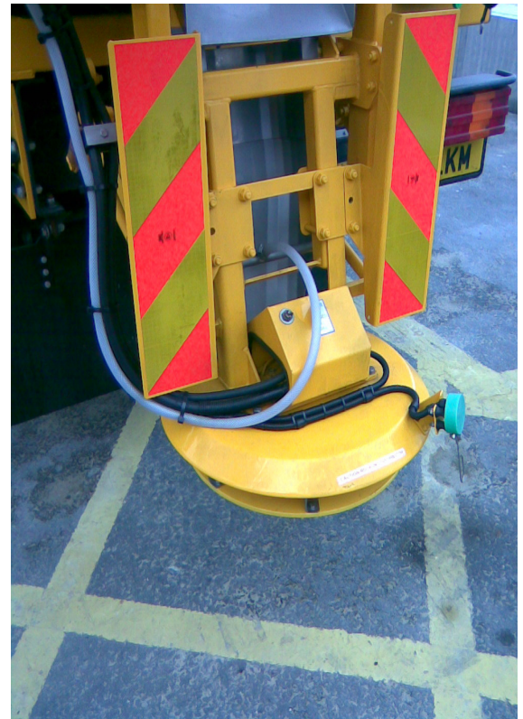
Figure 4.1 Modified Gritter Vehicle showing pre-wet tanks (left hand side) and application dish (right hand side)
