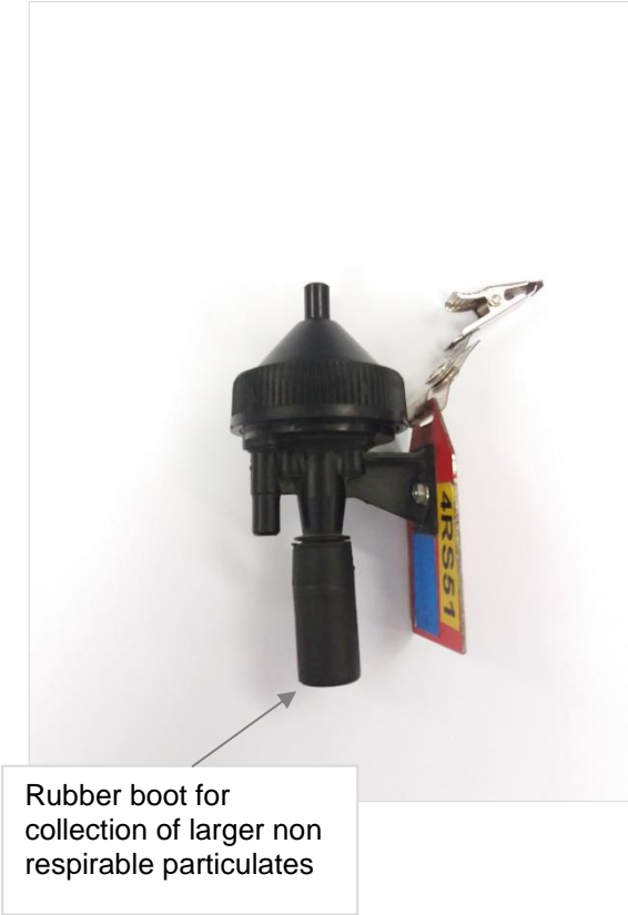
Figure D. Examples of air samplers used for collecting airborne dust.
