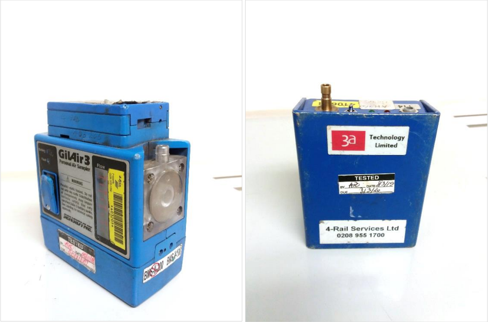
Figure D. Examples of air samplers used for collecting airborne dust.
