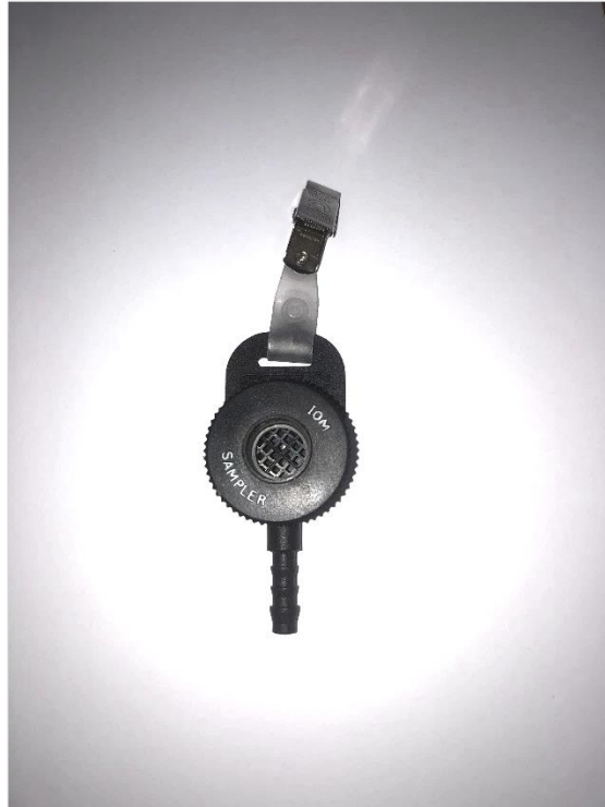
Figure B. Impactor Heads to monitor PM 2.5 and PM 10 aerodynamic diameter dust fraction size.
