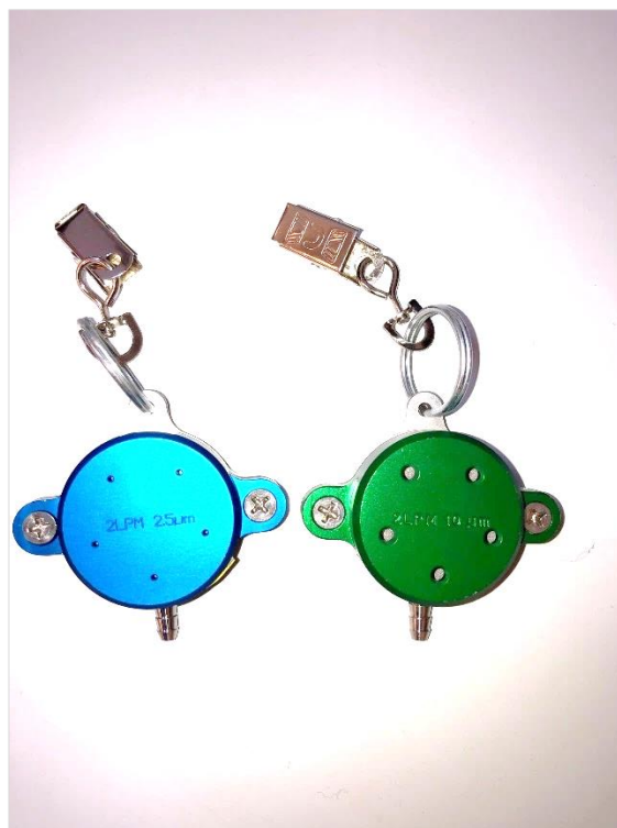
Figure B. Impactor Heads to monitor PM 2.5 and PM 10 aerodynamic diameter dust fraction size.
