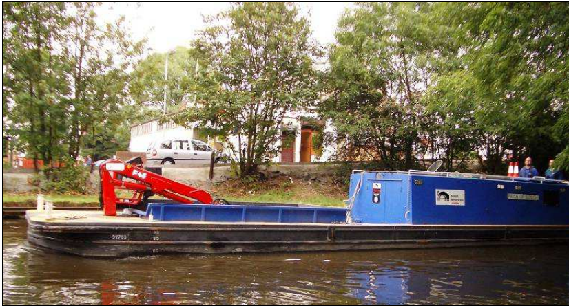
Figure 15: Barge fitted with telescopic crane
