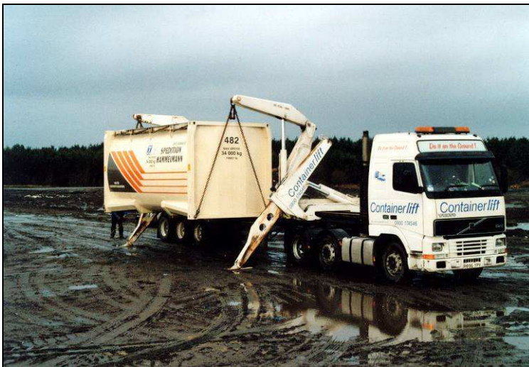
Figure 20: Container being unloaded from Containerlift vehicle
