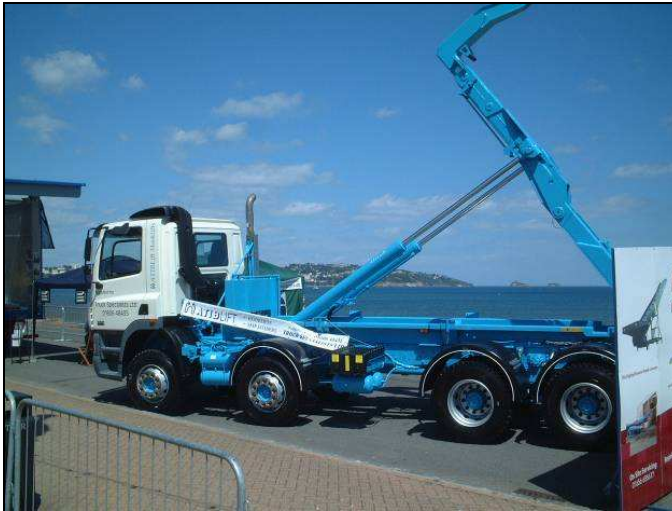
Figure 9: 32 tonnes hooklift vehicle
