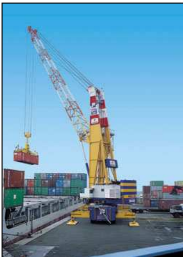
Figure 12: Large mobile port crane
