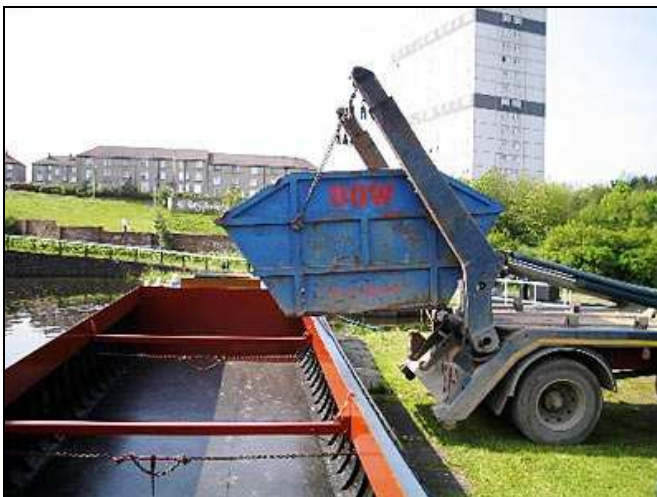
Figure 8: Transferring a skip to a barge using a skip lorry
