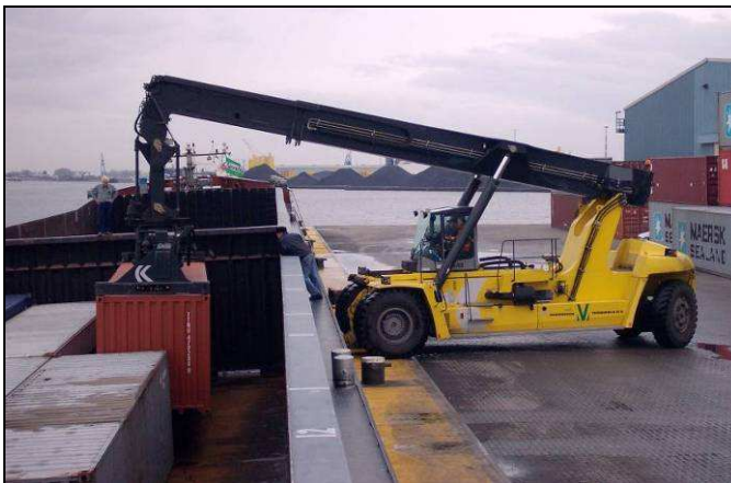
Figure 18: Reach stacker loading a barge
