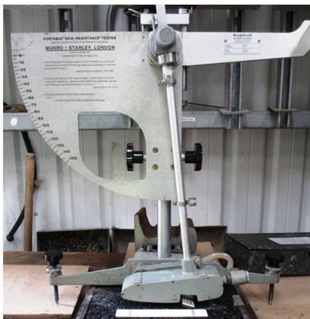
Figure 3-1: The Portable Skid Resistance Tester
