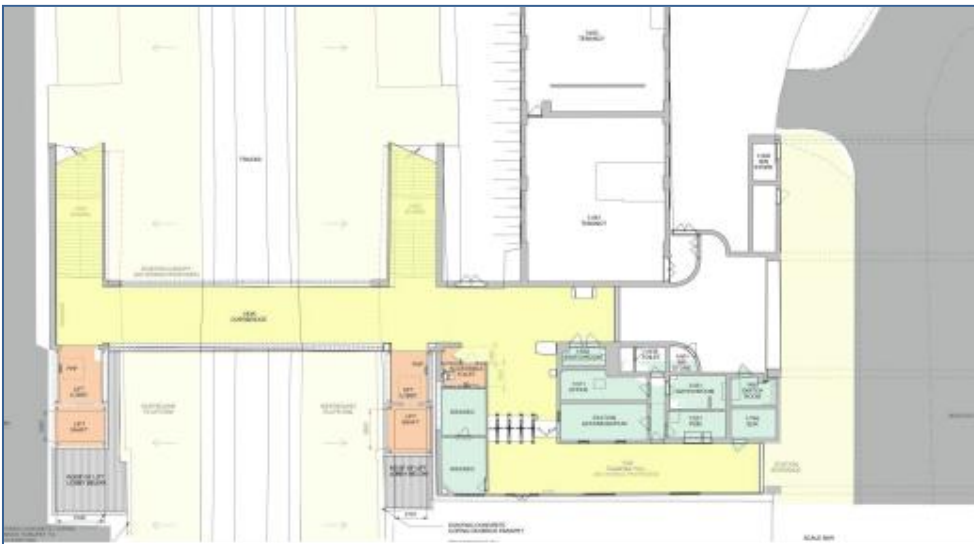
Newbury Park station - Proposed location of new lifts constructed off rear of existing over bridge
