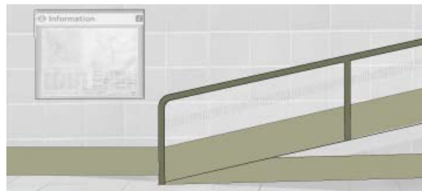
Low-level colour contrast on walls
