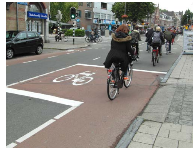
ASLs with lead-in lanes are also used in other countries – as in this example from Utrecht
