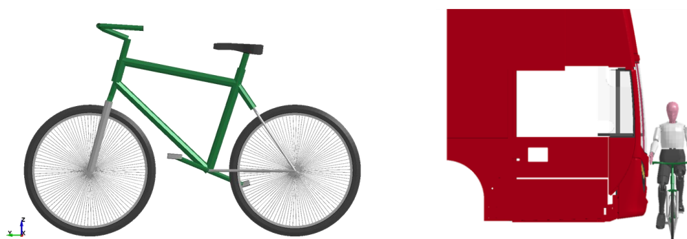
Figure 25: The setup used for the simulation of bus versus cyclist collisions; bicycle model (left), bicycle with seated dummy in front of bus (right)
