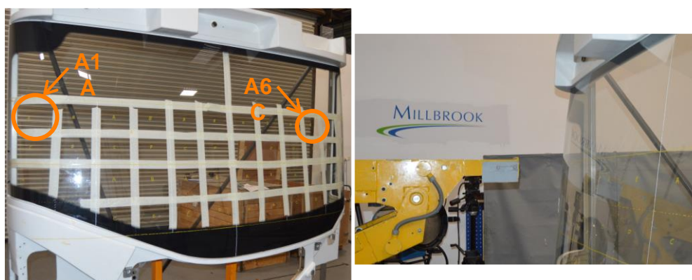
Figure 33: Set up of APROSYS HVAI impact zones (left) and the wraparound windscreen impact test against the A1A impact position (right)
