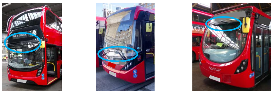
Figure 8: Various windscreen wiper mounting positions for double and single deck buses
