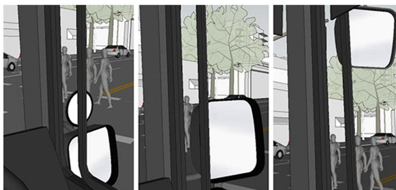
Figure 17: A bus driver's view of a pedestrian crossing with three different mirror configurations: inverted mount (left); medium mount (centre); high mount (right) (Leverette, 2013).
