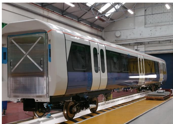
First assembled carriage mounted on its bogies
