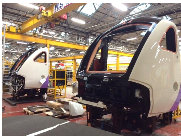
Fit-out of driving cab sub-assemblies prior to bolting to car
