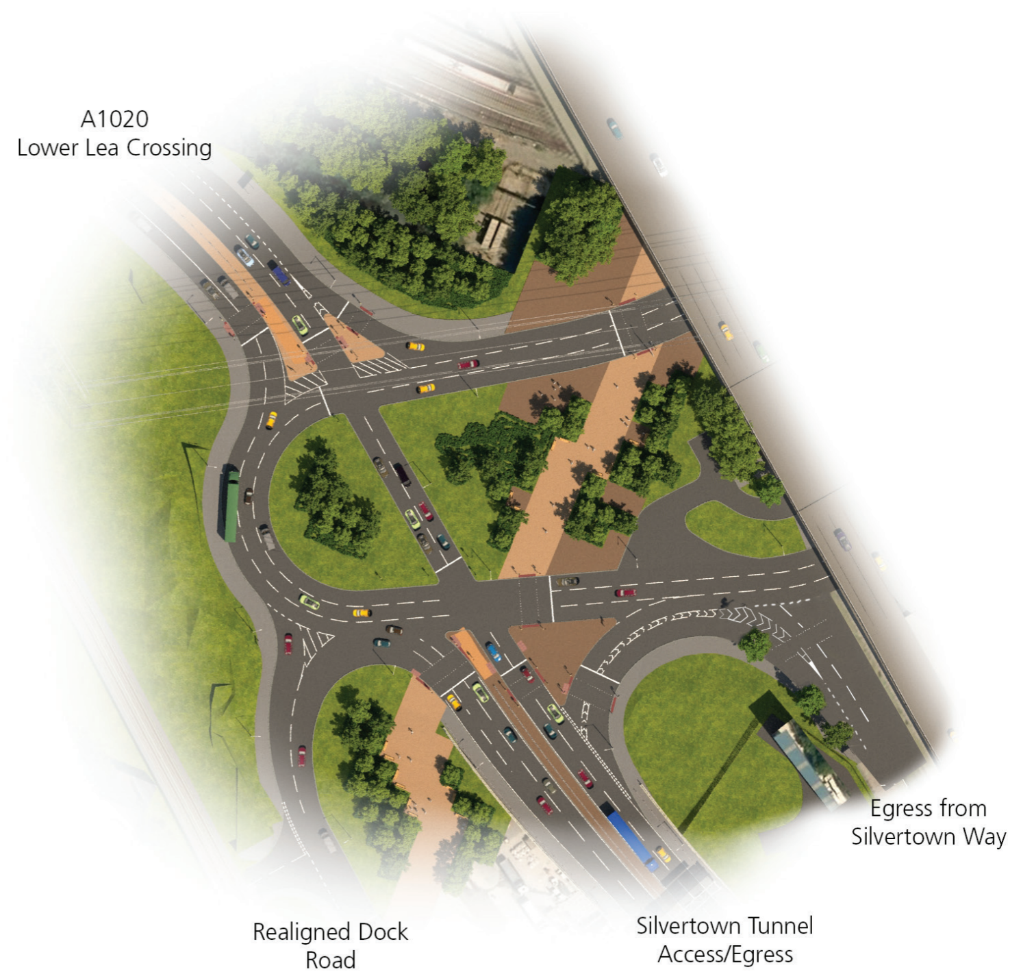
Figure 4.1 – Illustrative birdseye view of the modified Tidal Basin Roundabout
