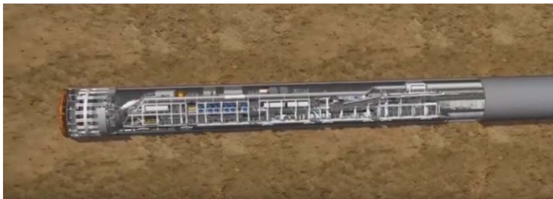
Figure 1 Cutaway view of a large diameter tunnel boring machine (Herrenknecht)
