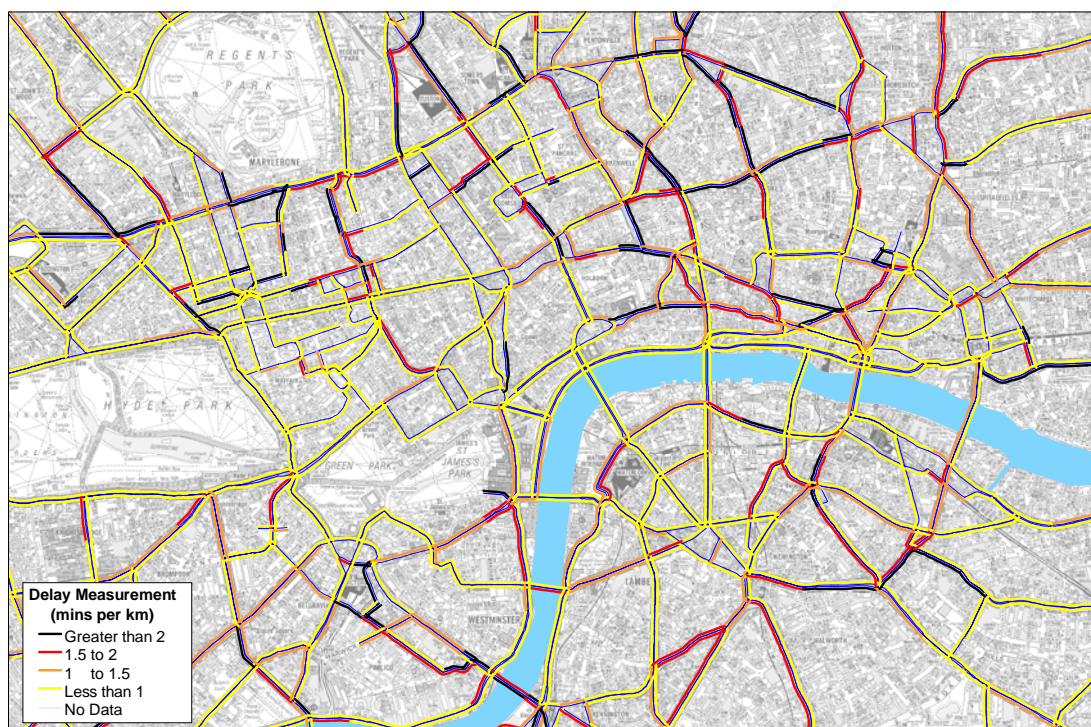
Figure 3.10 Example plot using ITIS satellite-based congestion data, within and around the central London congestion charging zone, 07.00 to 10.00 Monday to Friday, October 2003.
