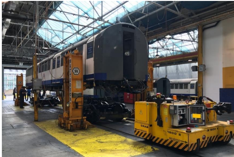
Figure 2: Overhaul of a Central line RAT
