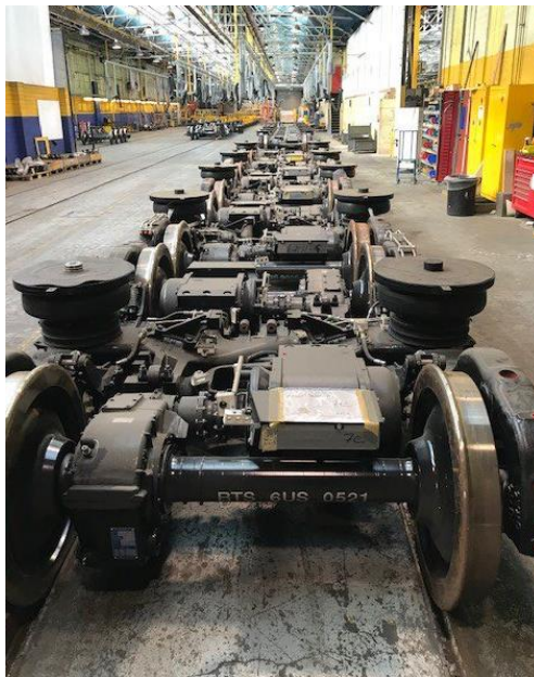
Figure 1: Metropolitan line fleet bogies being prepared for programme lift
