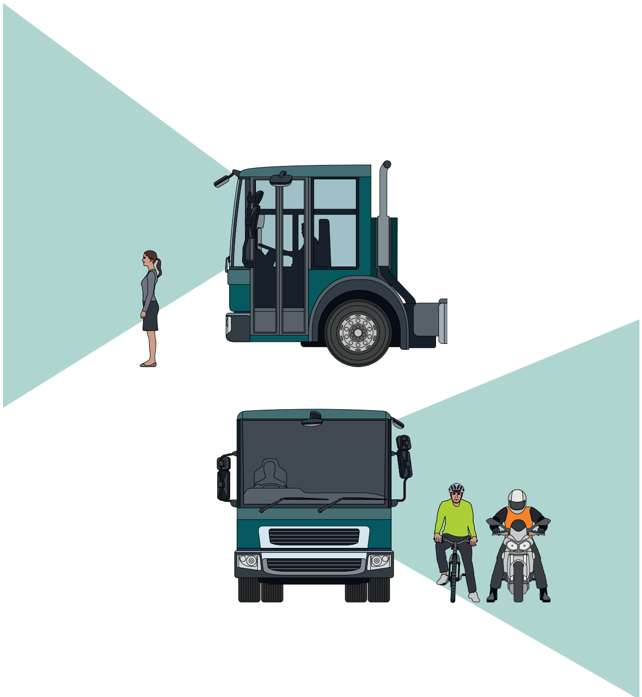
Figure 14: High vision HGVs increase drivers' ability to see other road users directly through their cab windows
