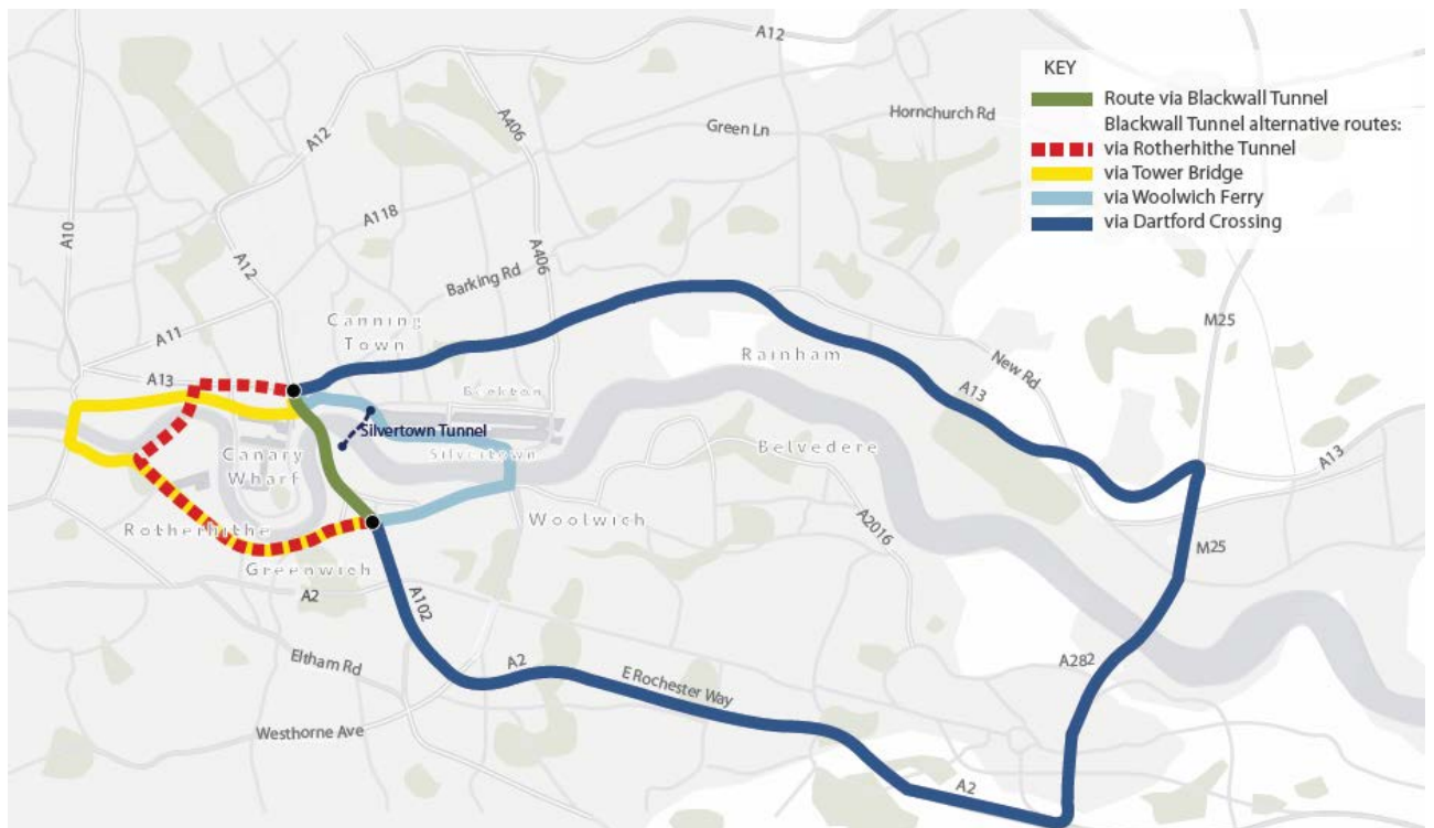
Figure 5-1: Blackwall Tunnel diversion routes
