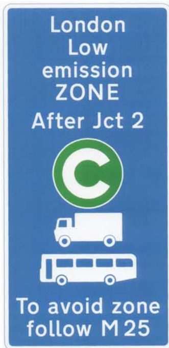
Sign Type 1 Advance Informatory
