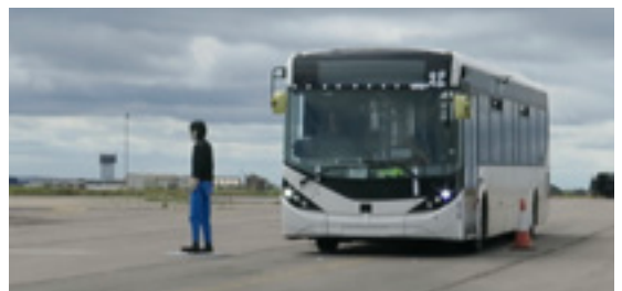
Advanced Emergency Braking (AEB) applies braking (if the driver is unresponsive) to avoid the pedestrian.
