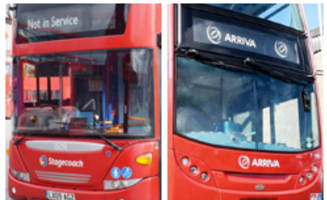
Windscreen wiper protection must be provided, unless they are located at the top of the screen out of harm’s way.
