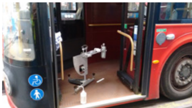
Slip resistance in use was investigated; measurements will use samples for new buses.
