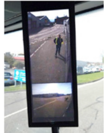
A Camera Monitor System (CMS) can replace the wing mirror and help to reduce blind spots.
