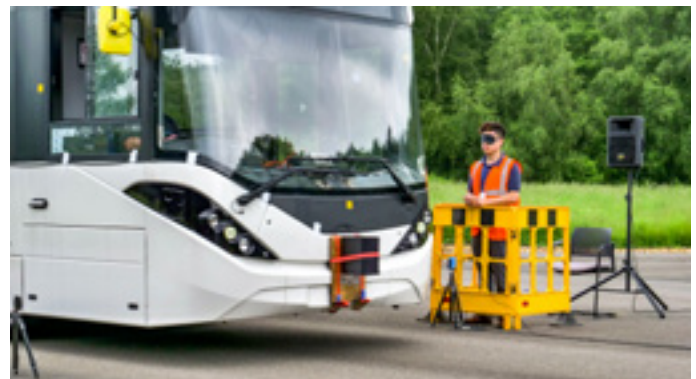
Acoustic conspicuity trials showed a greater effectiveness of the sound coming from the front of the bus.
