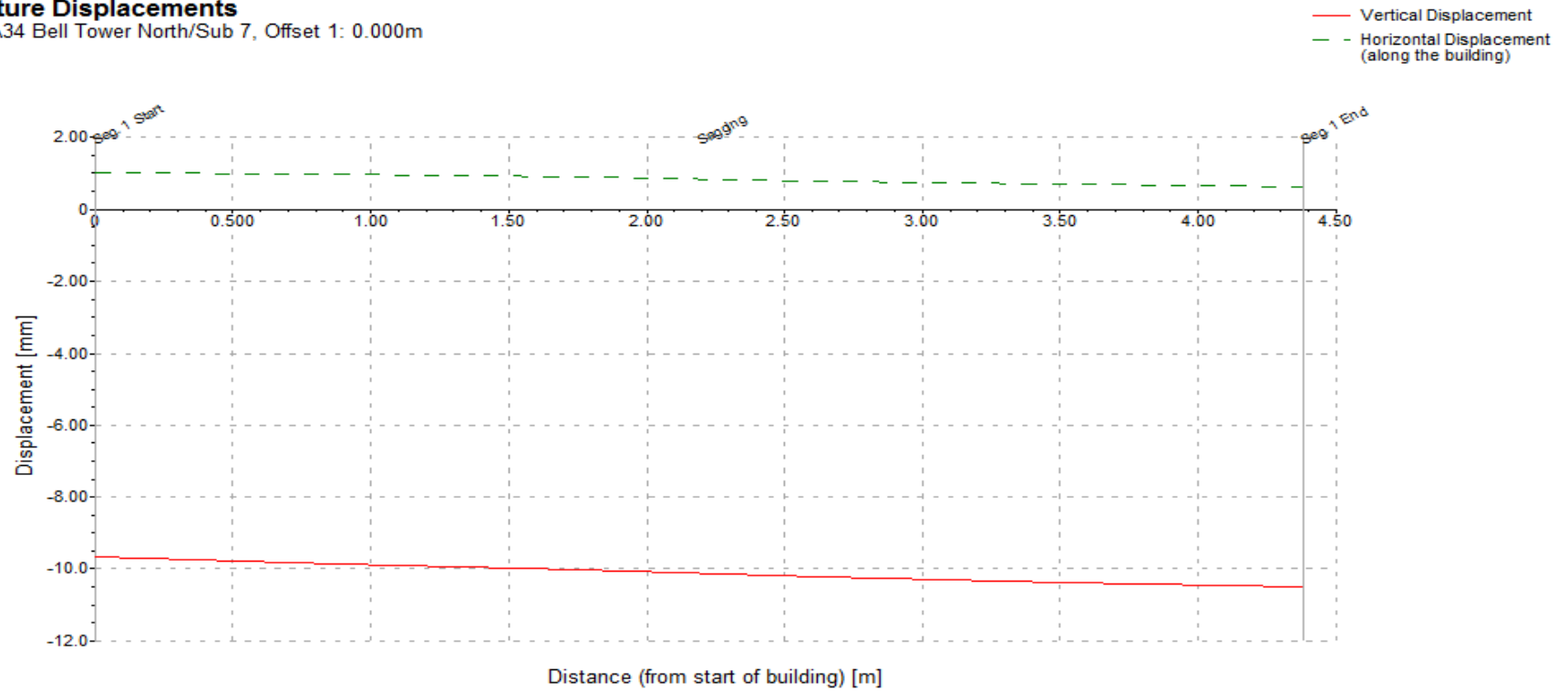
Figure 7: Building displacement at founding level (Bell Tower) at stage 1 (line 4) of worst case for tensile strains
