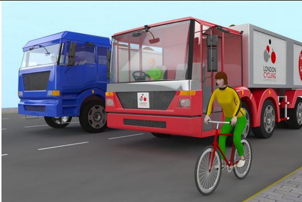
Figure 36: Redesigned lorry cab for improved direct vision of cyclists (London Cycling Campaign image)
