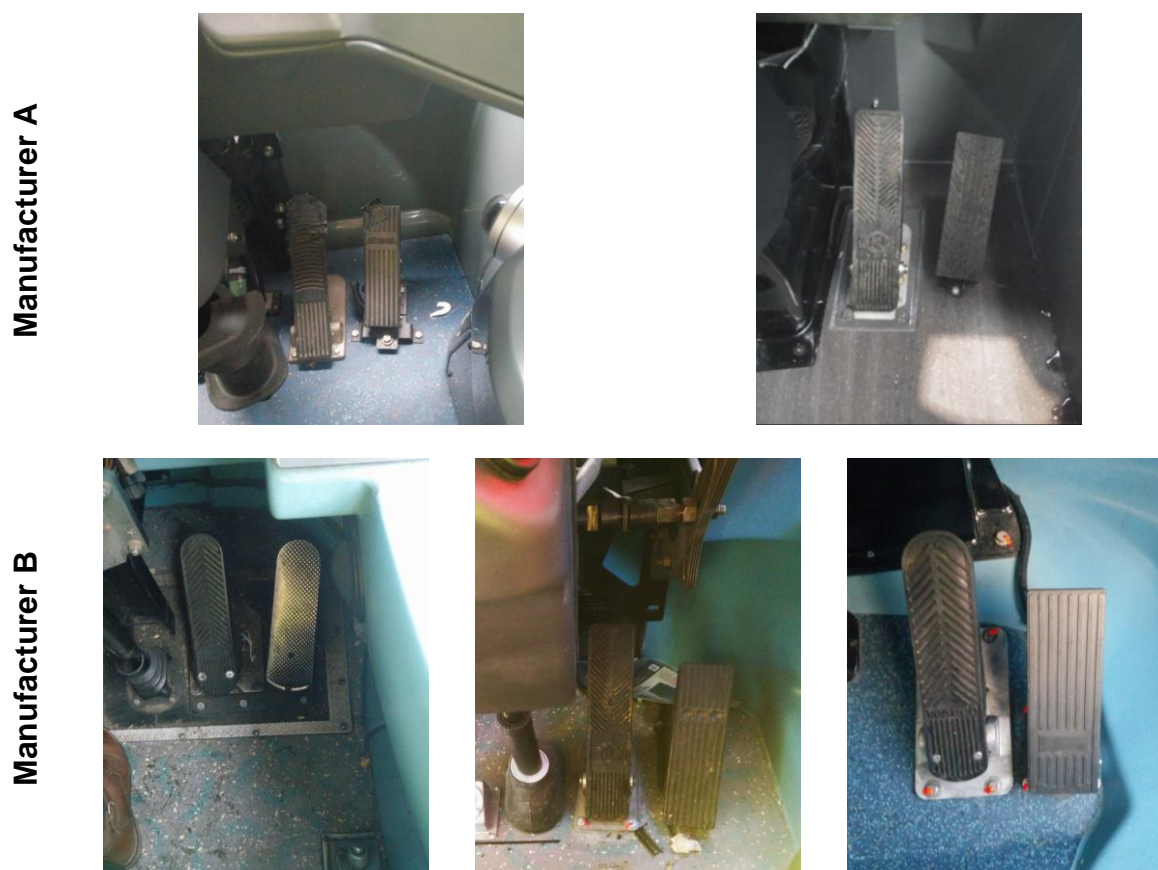
Figure 3: Two pedal configurations from Manufacturer A (top) – Three pedal configurations from Manufacturer B (bottom)
