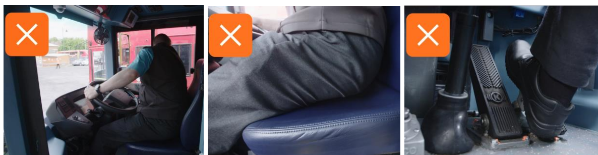
Figure 7: Arriva training video on pedal application error – impact of upper body movements on lower body parts when checking the blind spots
