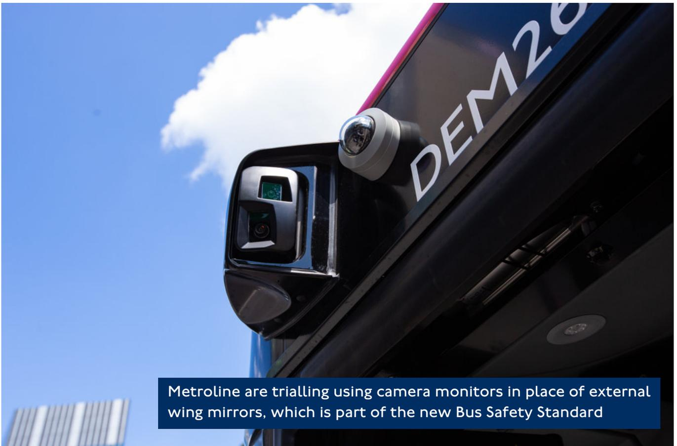
**Metroline are trialling using camera monitors in place of external wing mirrors, which is part of the new Bus Safety Standard**
