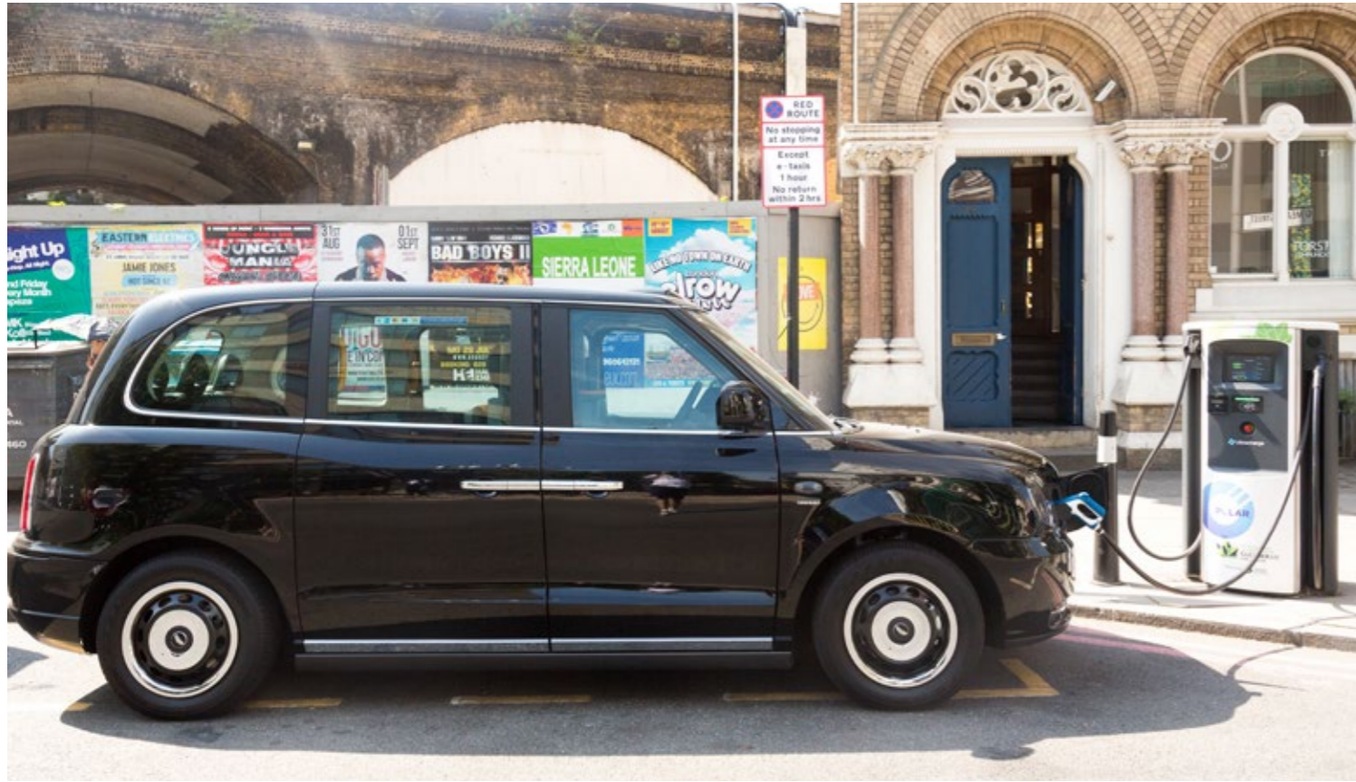
Image 25 LEVC Taxi charging at rapid charge point
