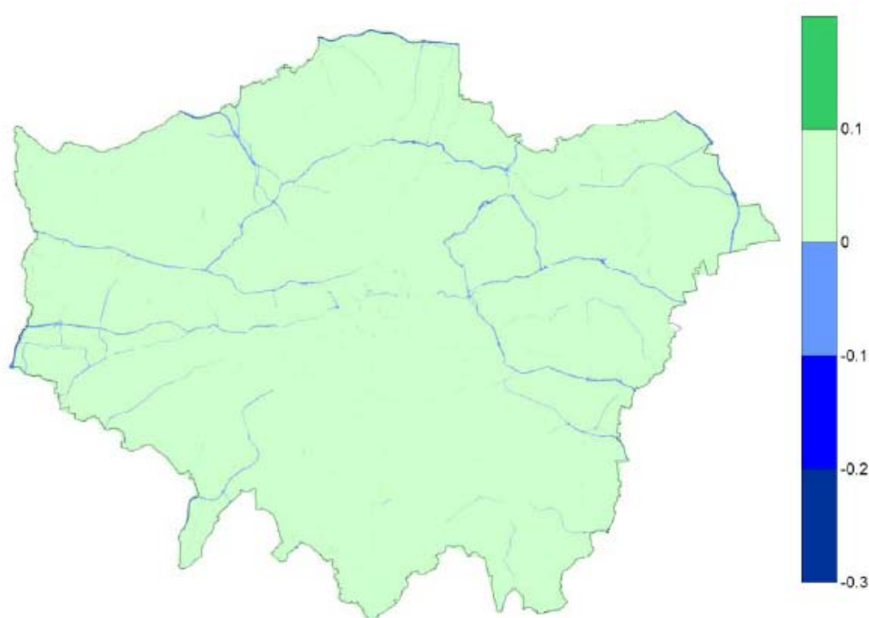
Figure 3: Deferral of LEZ Phase 3 from October 2010 to January 2012: Predicted impact on annual mean NO 2 concentrations in 2011
