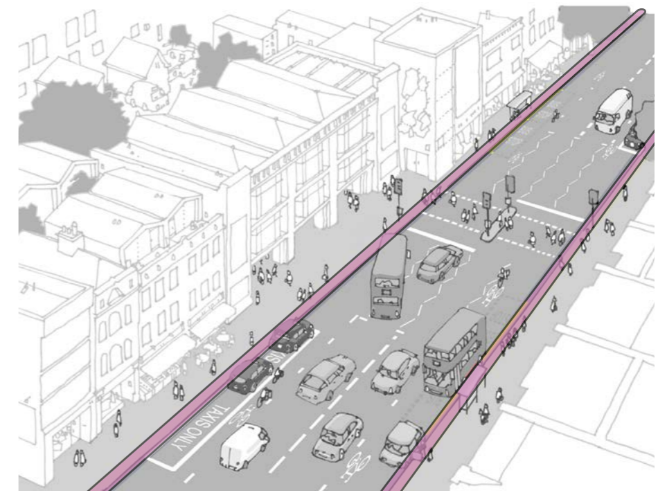
Figure 5.11. The kerb line
