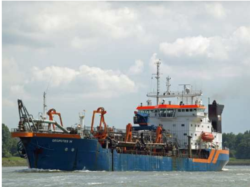
Trailing suction hopper dredger
