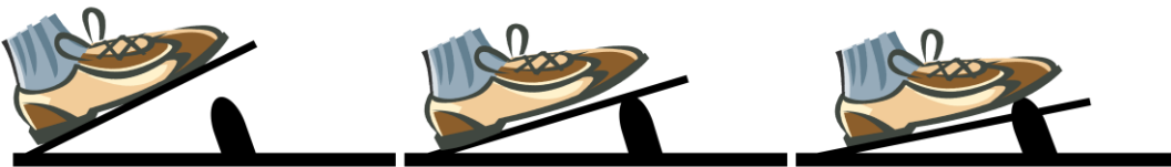
Figure 11 – Tactile protrusion giving feedback to driver’s foot when fully accelerating
