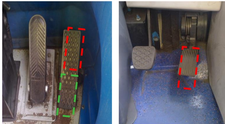
Figure 4 – Examples of Differentiation through Changing the Size of the Pedals (coloured boxes indicate different size/positioning options)
