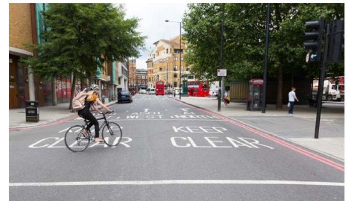
Keep clear markings allow space for cyclists to cross
