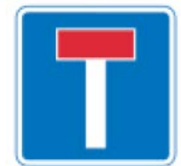
816 – no through route for vehicular traffic
